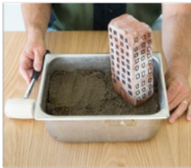
Liquefaction simulation of the potential behavior of buildings during an earthquake.
